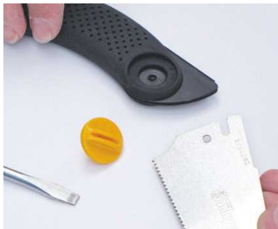
...and simply unscrew and slide out the blade
